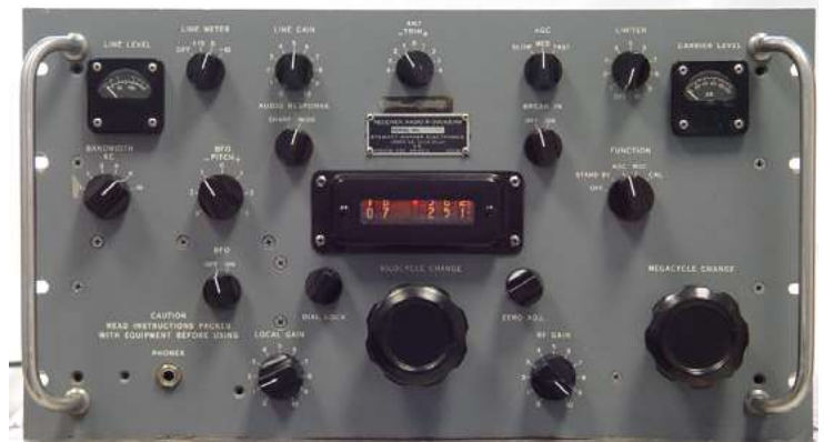
Weighing 65 pounds, the R-390A/URR was a go-to receiver for many shortwave listeners for decades. Above is the Stewart-Warner Electronics version. (Courtesy: Universal Radio)
